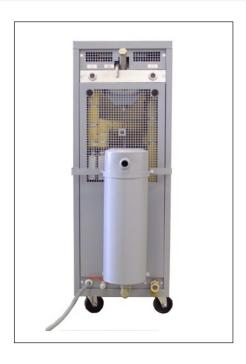
The condensing divertor protects from hot steam, which comes out through the water outlet when the cooling function is required by high temperatures of oil. Hot steam can damage the water soil pipes out of PVC and damage hoses.
